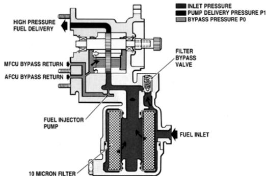
**Figure 7-37 Engine Driven Fuel Boost Pump**
