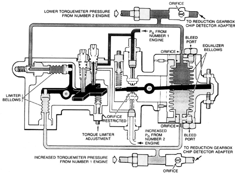
**Figure 7-43 No. 1 Engine Torque Higher than No. 2 Engine Torque**
