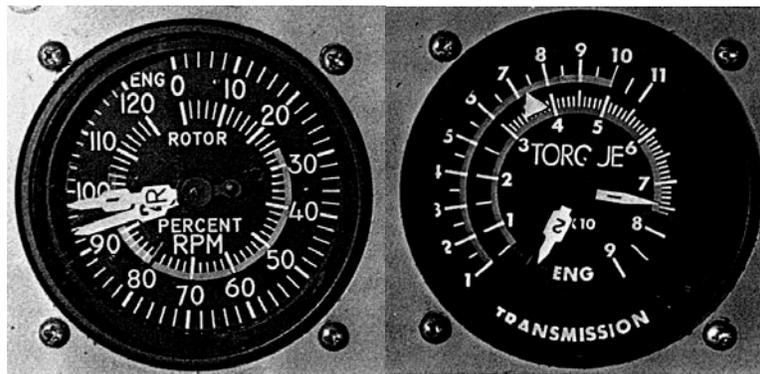
**LOW-SIDE FCU FAILURE DURING LOW POWER DEMAND**
