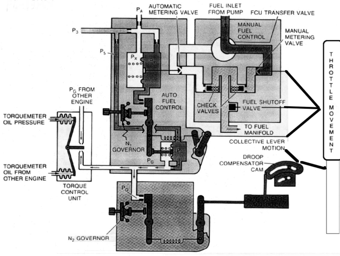
**Figure 7-48 Fuel Control Manual Mode**
