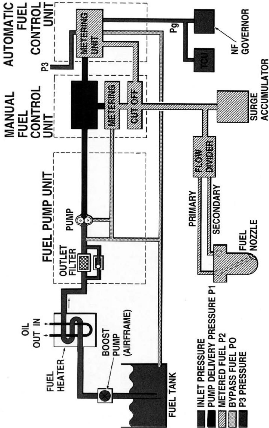
Figure 7-31 Fuel System Schematic
