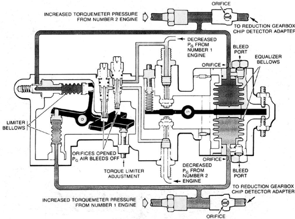
**Figure 7-44 Torque Limiting**
