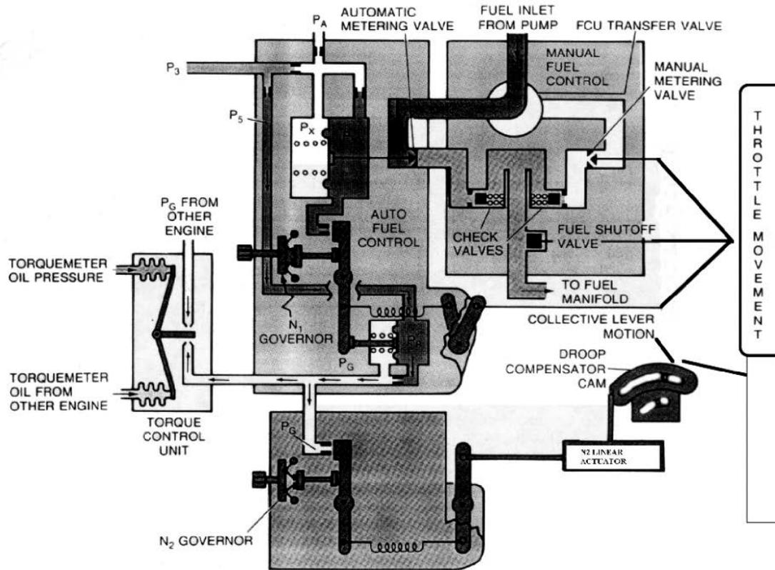
**FIGURE 7-39 Fuel Control Automatic Mode**
