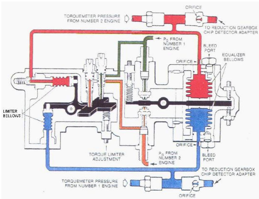
**Figure 7-42 Torque Control Unit Diagram**
