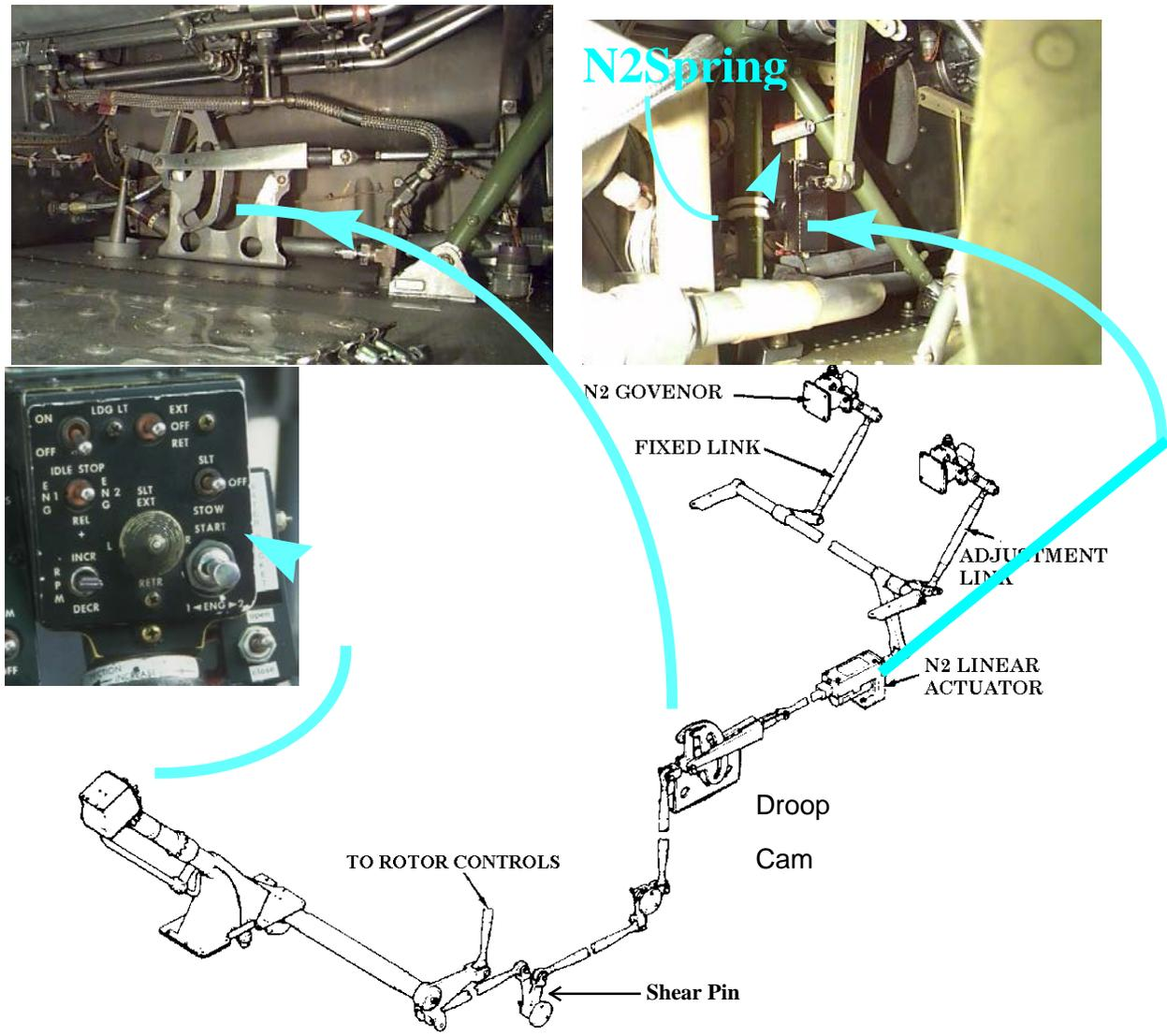
**Figure 7-40 RPM Beep Switch and Droop Compensator**
