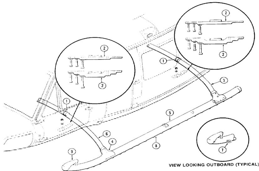
**Figure 2-16 Skid Landing Gear**
