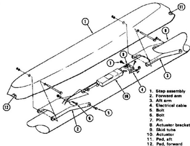
**Figure 2-17a Emergency Floats (top) and Passenger Step Kit**
