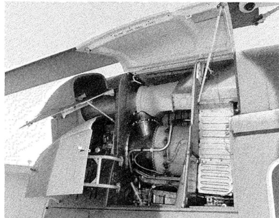
**Figure 2-14 Engine Deck**
