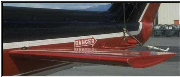
Figure 2-19 Synchronized Elevators
