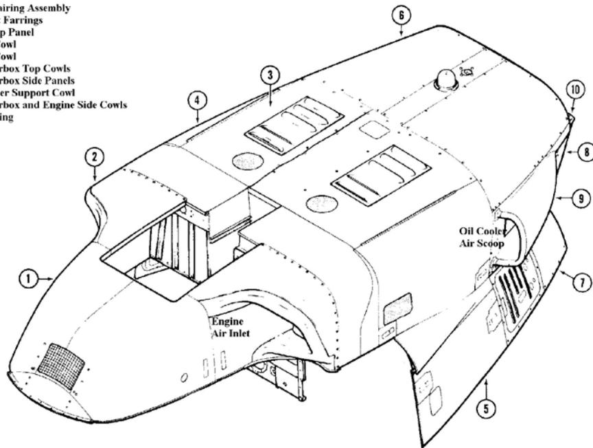
**Figure 2-15 Transmissions and Engine Cowling**
